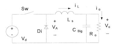
b. (3 points) Find and sketch the diode voltage waveform. Label its maximum voltage, its minimum voltage, and the times that switching occurs during at least one switching cycle.
