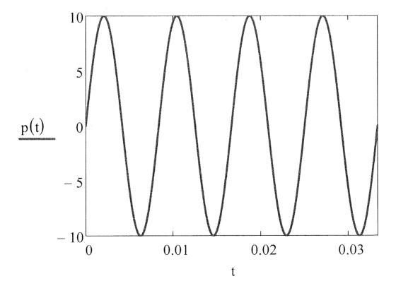
Example Double Frequency Power Term. For a voltage of 10  $cos(\omega t)$ Volts and a current of  $2cos(\omega t-\theta)$ Amps, find the power as a function of time. Vary the power factor over its range to see if there is any effect on the power output.
