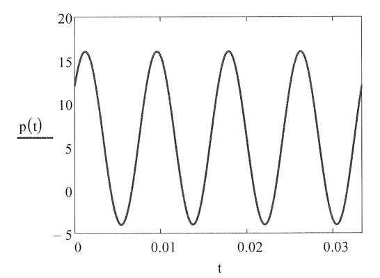
Example Double Frequency Power Term. For a voltage of 10  $cos(\omega t)$ Volts and a current of  $2cos(\omega t-\theta)$ Amps, find the power as a function of time. Vary the power factor over its range to see if there is any effect on the power output.
