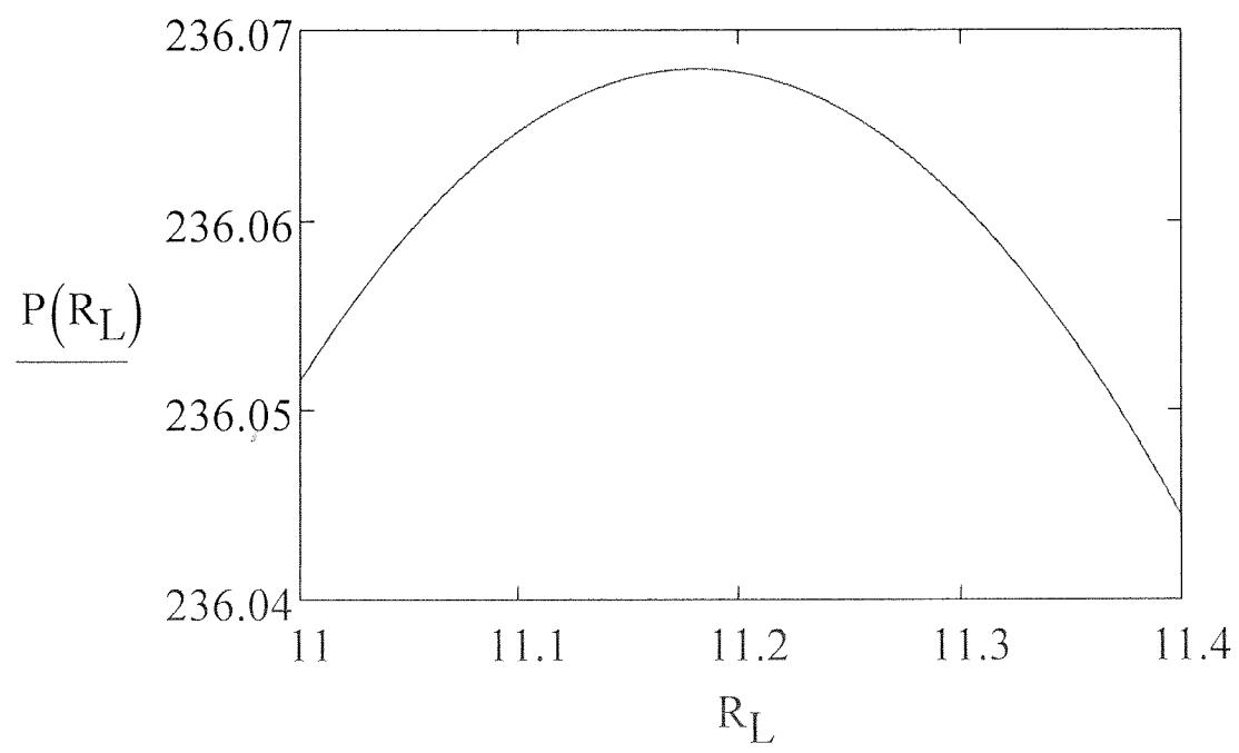
Max Power Transfer Example. For a circuit with a 100V AC source and a  $(10+j5)\Omega$  source impedance, find the output power as a function of load resistance for a resistance only load.
