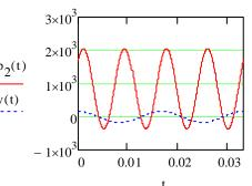
The average value of this power waveform is about 800 Watts.
