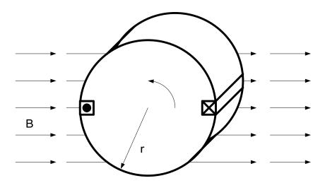
b. (3 points) The conductor is connected to a 0.05 Ohm resistor. For the voltage that you found in part a and the current direction as shown, determine the magnitude and direction of the induced torque. If you didn't find a voltage in part a, make one up.
