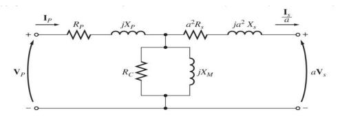
Below is the transformer model referred to Secondary Side.
