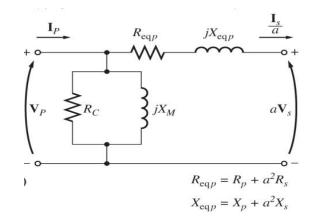
• Simplified equivalent circuit referred to secondary side:
