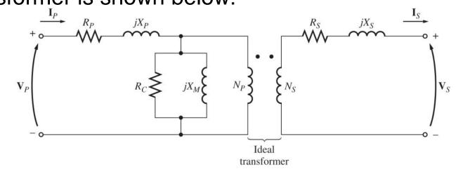
The equivalent circuit may be simplified by *reflecting* impedances, voltages, and currents from the secondary to the primary as shown below:
