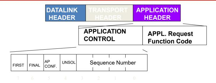
FIN = Final Indication 1 = FINal Fragment in sequence 0 = More Fragments Follow FIR = FIRst Frame 1 = First Fragment In a Sequence 0 = Not The First Fragment AP CONF. = Application Confirm 1 = Ap Layer Confirm Expected 0 = No Ap Layer Confirm Expected.
