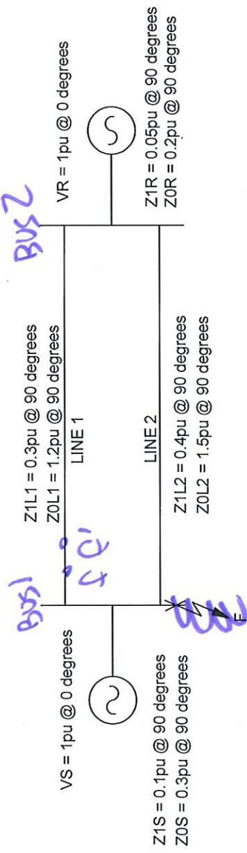
$$Z_{1S} := j0.1 \text{pu} \quad Z_{1R} := j0.05 \text{pu} \quad Z_{0S} := j0.3 \text{pu} \quad Z_{0R} := j0.2 \text{pu}$$
