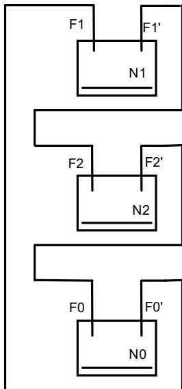
$$I_1 := \frac{V_{\text{equiv}}}{Z_{1FF'} + Z_{2FF'} + Z_{0FF'}} \quad I_1 = (0.2 - 0.12i) \cdot \text{pu}$$
