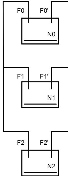
$$I_1 := \frac{V_{\text{equiv}}}{Z_{1FF'} + \left( \frac{1}{Z_{2FF'}} + \frac{1}{Z_{0FF'}} \right)^{-1}}$$
