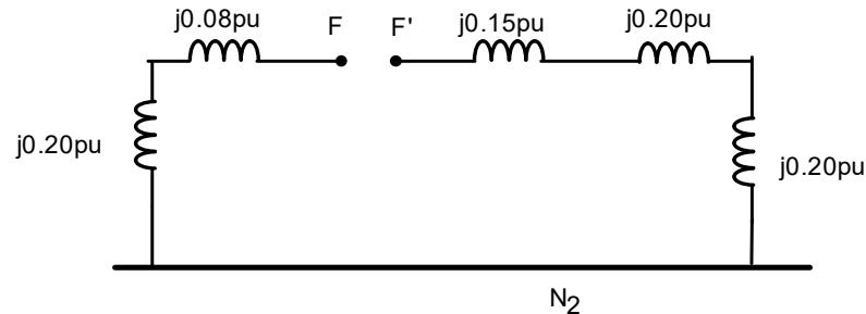
Find total impedance counterclockwise around loop from  $F$  to  $F'$
