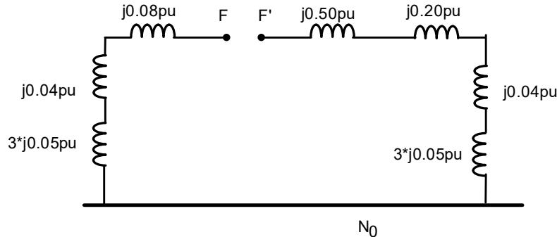
Find total impedance counterclockwise around loop from  $F$  to  $F'$
