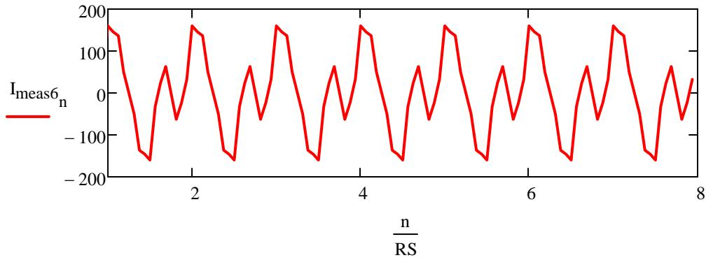
$$\text{Phasor6}_v := \frac{1}{\sqrt{2}} \left( \text{COSF}\left(RS, I_{\text{meas}6}, v\right) + j \cdot \text{COSF}\left(RS, I_{\text{meas}6}, v - \frac{\pi}{4}\right) \right)$$
