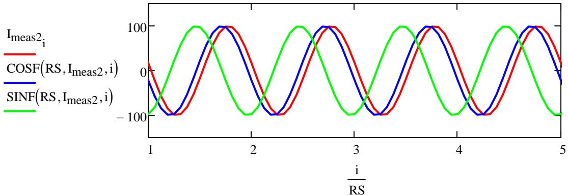
$$\text{Phasor2}_i := \frac{1}{\sqrt{2}} (\text{COSF}(RS, I_{\text{meas2}}, i) - j \cdot \text{SINF}(RS, I_{\text{meas2}}, i))$$
