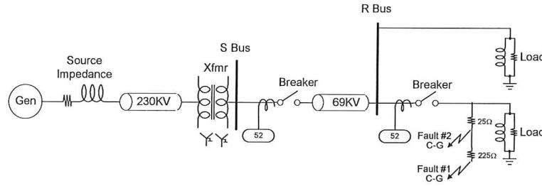
250Ω resistive fault is initiated at 8.3 ms and progresses to a 25Ω fault at 62 ms as can occur by a tree branch coming in contact with the wire.
