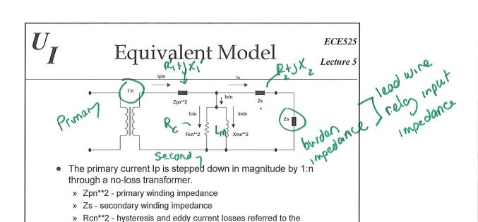
Xmn\*\*2 - magnetic reactance accounting for losses to establish flux
