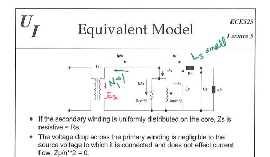
The secondary current is reduced by the shunting current of the exciting branch. The greater le the less accurate is represents ip.
