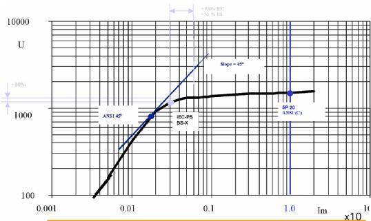
The knee point voltage is the highest exciting voltage generated by a **symmetrical** secondary short circuit current on which the flux in the CT will not reach the saturation flux.
