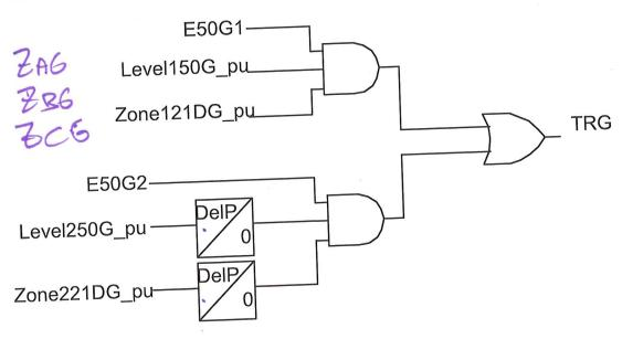
Phase distance element logic diagram:
