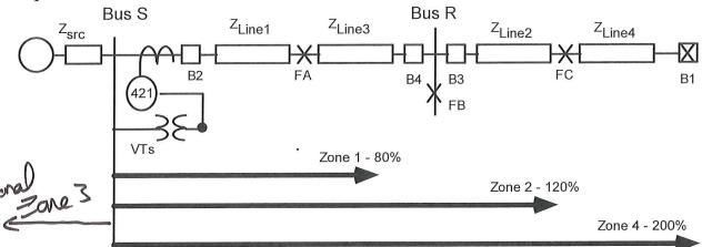
Case 1: Set the phase and ground distance elements in the SEL 421 at Bus S to provide instantaneous under-reaching tripping against faults (3-phase, LL, SLG) at FA.
