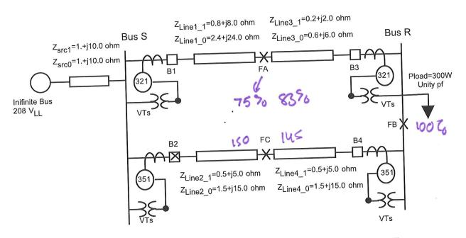
Please Note: breaker B2 is open, distance relay SEL 321 is used to provide 2-zone distance protection.
