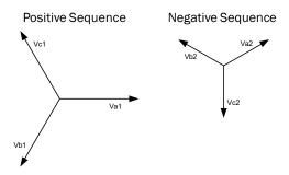
All of the phasors rotate counter-clockwise. It is the sequence that changes.
