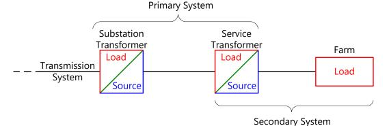
Current circulates between a source and load.
