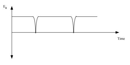
Case II: Run current through a stationary loop in the magnetic field.
