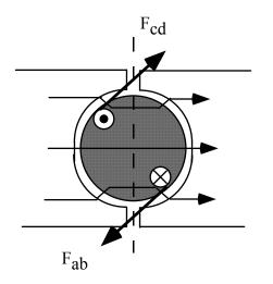
Now the current interacting with the magnetic flux density (or flux) produces a force on the wire. Since the current in segments ab and cd are in opposite directions, two forces are produced that will try to rotate the wire loop.
