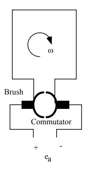
• Now connect the rings to a fixed electrical circuit and measure that voltage. Now the circuit connection to the commutator reverses at the same point where the voltage reverses, resulting in the voltage waveform below, which is a much better approximation of DC.
