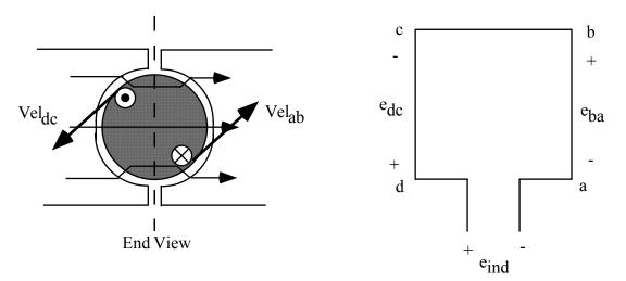
Assuming the flux divides equally, whenever the longitudinal segments (ab and cd) of the loop will see equal flux. The velocity of these segments (ab and cd) is defined as shown, and it tangential to the surface of the rotor at the location of the loop. From Faraday's Law
