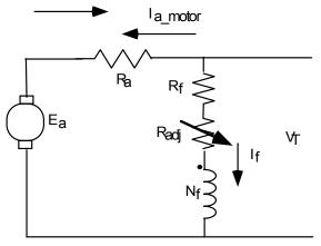
• In the generator case,  $V_t$  will depend on  $E_a$ , so it will be necessary to vary  $I_f$  to keep the terminal voltage at a desired level.
