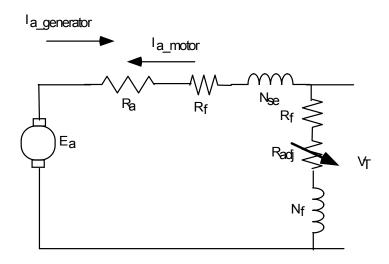
• Shunt field can be connected between series field and armature winding (short shunt) or between the series field and terminal voltage (long shunt).
