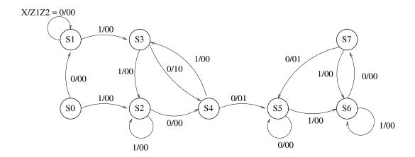
**3.** Design a Moore network state diagram for a state machine with one input and one output. A sequence of 101 toggles the output between 0 and 1. Note that the sample sequence changes the output *after* the 101, not at the same time as the last 1. Can start in either S0 or S1.
