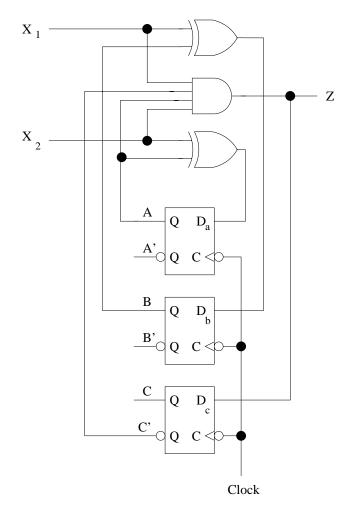
2. (8 pts) The sequential circuit below yields an output sequence of Z = 11011111 when you apply the input sequence X = 01101010. What is the starting state A?
